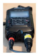
Plug the side of the cable with the big jack plug into the the same jack on the Zoom where you would normally plug in the mic. The Zoom is conveniently outfitted with **combination-jacks** for **XLR** as well as **jack plugs**.
