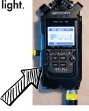
Phantom power means that the mic is getting electricity from the recorder and does not need extra batteries.
